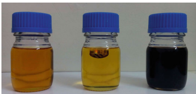
Fig. 1 Karanja oil ( left ), Karanja oil methyl ester ( centre ) and Karanja oil based biolubricant ( right )
