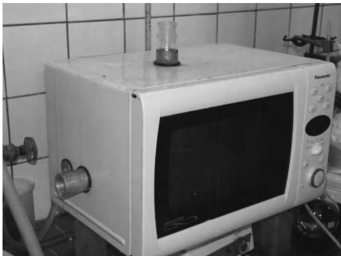
Figure 3.1 Modified domestic household microwave oven. Inlets for temperature measurement by IR pyrometer (left side) and for attaching reflux condensers (top) are visible. A magnetic stirrer is situated below the instrument.
