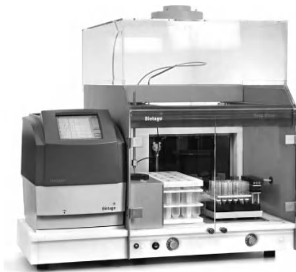
Figure 3.9 Biotage Syro Wave: fully automated microwave and parallel peptide synthesizer.
