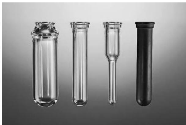
Figure 3.5 Monowave 300 vessel types: glass vials 6.0–20, 2.0–6.0, and 0.5–2.0 mL; and silicon carbide vessel 2.0–6.0 mL (left to right).
