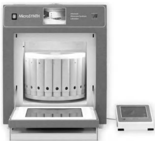
Figure 3.29 Milestone MicroSYNTH labstation with SafeVIEW system.
