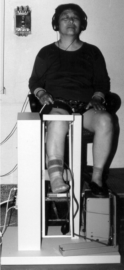
Fig. 2. Customized apparatus used to test passive motion sense of knee joint.
