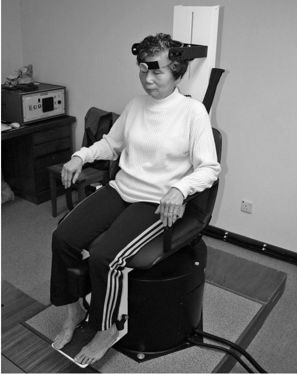
Fig. 3. Fixation of the subject and experimental set-up for whole head-and-body rotation using a rotational chair.
