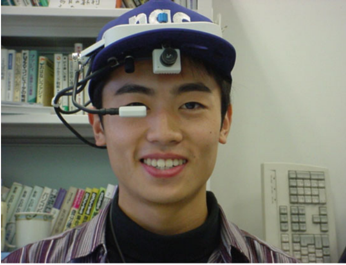
Fig. 11.2 Eye-gaze equipment. Source: Okubo et al. (2006)
