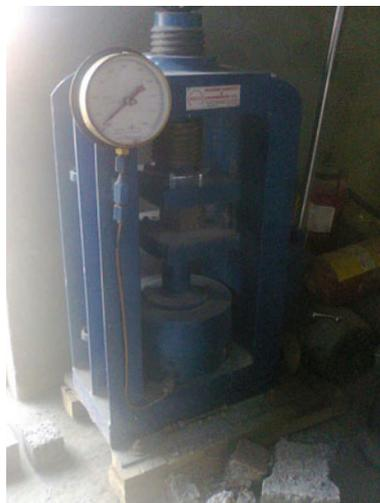
specimen takes place is then recorded, and compressive strength of the cube specimen is measured by using the formula;
