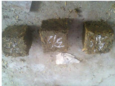
prepared by thoroughly bending the rice straws with the other starting materials: cement, fine and coarse aggregates, and water. Three specimen samples have been prepared for testing, by replacing the coarse aggregates by 10, 15, and 25% by weight. Proportioning of various constituents is shown in Table 10.2 and image of samples is as shown in Fig. 10.1.
