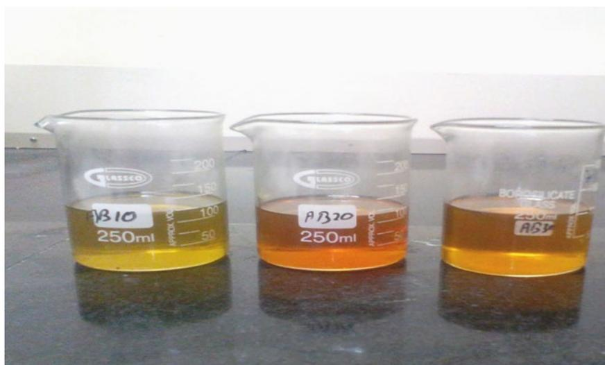
**Fig. 3.9** Argemone biodiesel blends AB10, AB20, AB30
