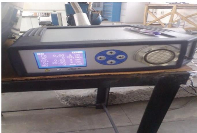
**Fig. 3.8** Exhaust gas analyzer
